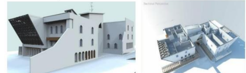
Positive and Negative pressure is induced by wing walls which helps in cross ventilation
