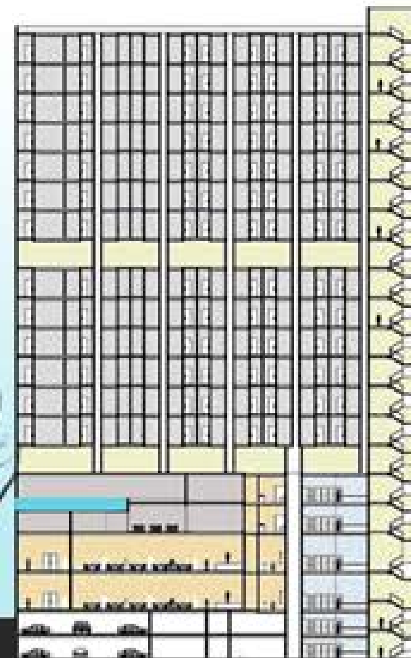
Longitudinal Section through stairs
