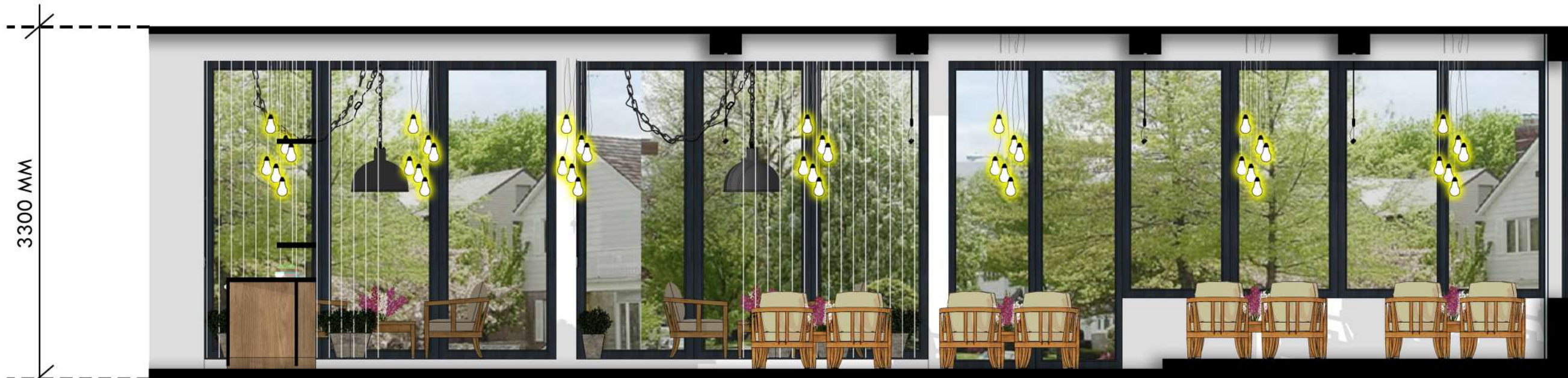
SECTION BB' SECTION SHOWING PARTITIONED SEATING AND USE OF FRENCH WINDOWS TO PROVIDE SUFFICIENT DAYLIGHTING AND NATURAL CONNECT.
