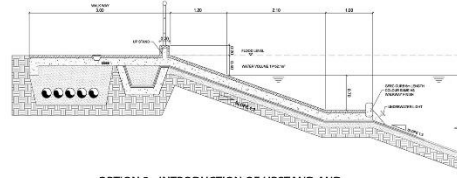
OPTION 3 - INTRODUCTION OF UPSTAND AND REDUCTION IN WATER LEVEL BY 100MM STORM WATER STORAGE CAPACITY 5658m 3
