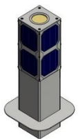
Stand-alone units with a height of 650mm on either side of a tree consisting of a housing, an AMMANU spot SL61 (can be tilted at an angle of 30 degree max.), a control unit, a battery, and a cover with integrated solar cells
