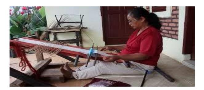
:- The young woman looked shrewd as her left hand was holding a small piece of wood about 1 meter long that wasused to lift a string of threads that were lined up neatly before her. One hand was ready to hold one end of a thin piece of black wood. Instantly the wood is inserted into a cavity formed from a series of threads of red and white are being raised.
