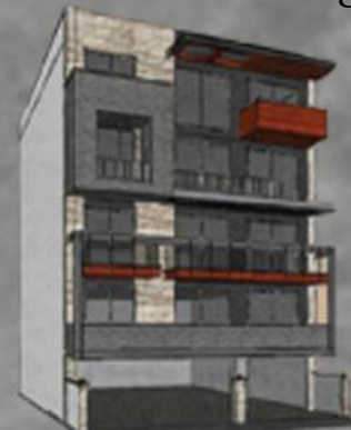
Adding elements like Vertical zigzag jali and 3 inch MD Girder and European jali Handrail
