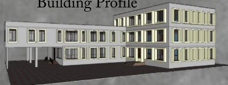
Created eggcrate window as shading device
