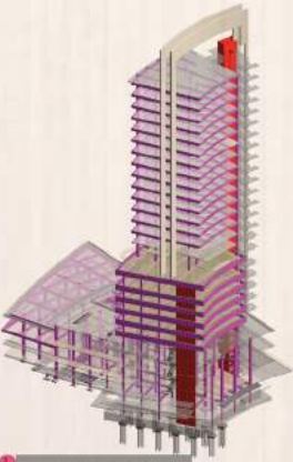
THE BUILDING IS COMPOSED OF TWO MAIN STRUCTURAL CORES AND A CONNECTING BRIDGE
